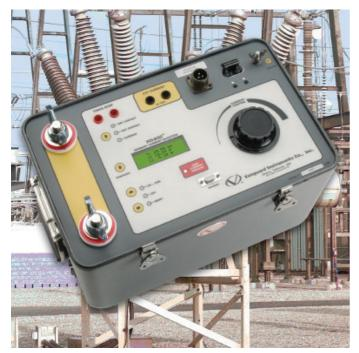
The VIC Model PCI-600 is a programmable, high-current source that is designed specifically for utility-substation applications. This alternating current (ac) test device is used primarily for injection testing of protective relays. This same device can also be used for testing thermal, magnetic and solid-state motor-protection relays and molded-case circuit breakers. The PCI-600 is versatile and can also be used in many other applications that require a high-current source.
