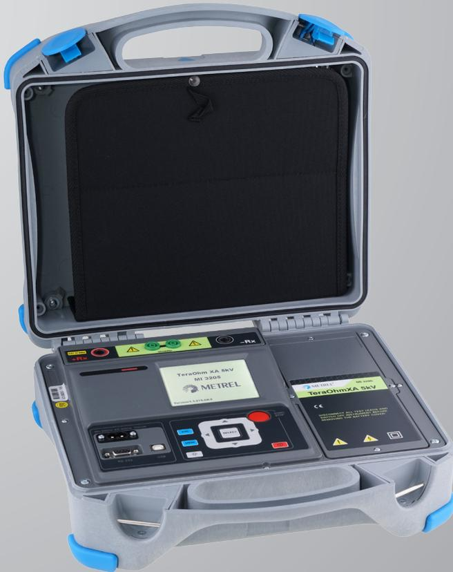
MI 3205 TeraOhm XA 5kV is a portable battery (Li-ion) or mains powered test instrument with excellent IP protection (IP65 case closed and IP54 case open), intended for diagnosing of Insulation Resistance by using high test voltages of up to 5 kV. It is designed and produced with the extensive knowledge and experience acquired through many years of working in this field.
