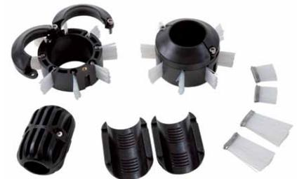
Each GatorCam4 system comes complete with a universal easy-fit brush skid set, that allows the 1" (25mm) camera to be used in pipes up to 4" (100mm) diameter and the 2" (50mm) camera in pipes up to 6" (150mm) diameter. Brushes can be conveniently replaced in seconds. Additional standard equipment may vary due to regional variations.
