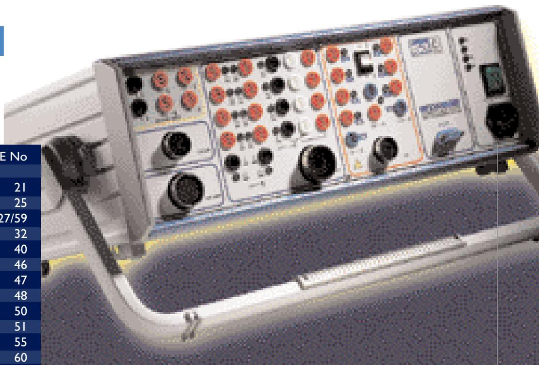
In addition to the above, the DRTS-3 has been designed to test the following equipment:
