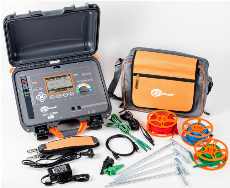
The Sonel MRU-120HD Ground Resistance Tester in weather proof hard case allows the user to take earth resistance measurements, using the 3-pole and 4-pole methods. Additionally, the MRU-120 offers selective earth resistance measurements, using an auxiliary clamp, meaning no influences from parallel earths or opening of junctions is required.
